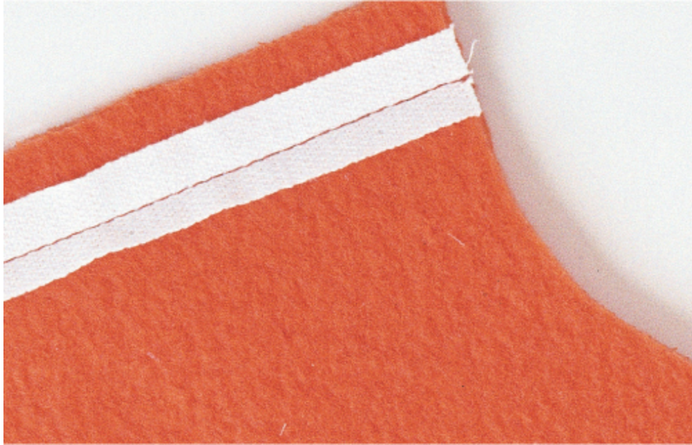
Knit fabric stabilized with stay tape
