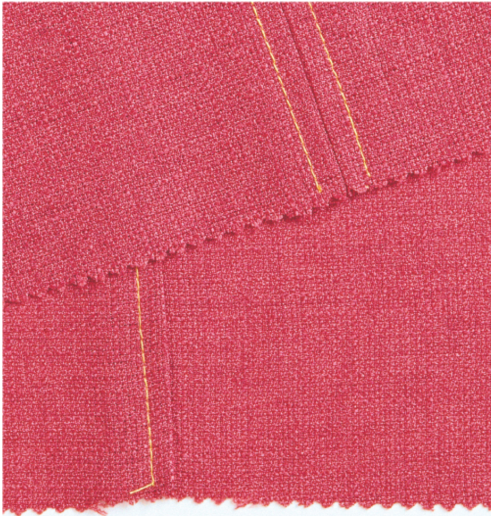
Topstitched seam and double topstitched seam
