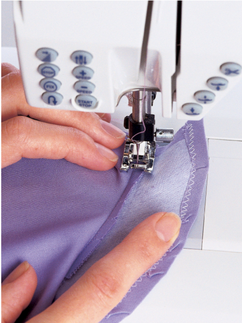
Understitching the seam allowances
