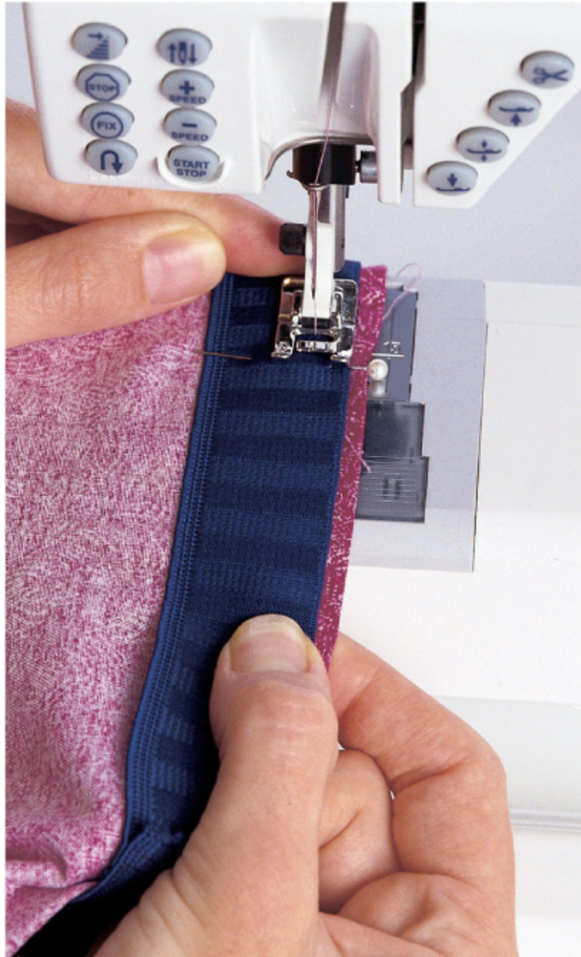
Stitching elastic with zigzag stitch to the wrong side of the top edge
