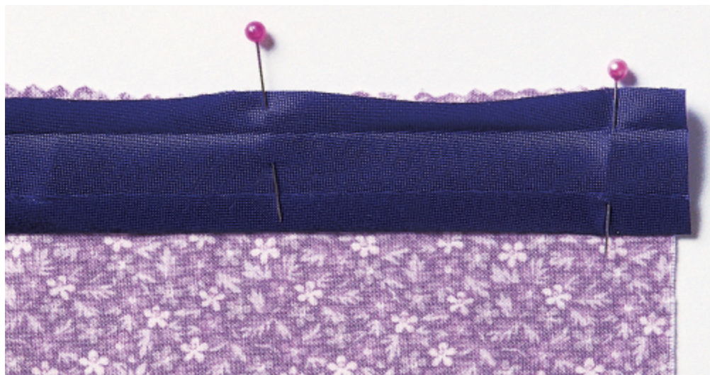
Bias binding being stitched to the fabric edge
