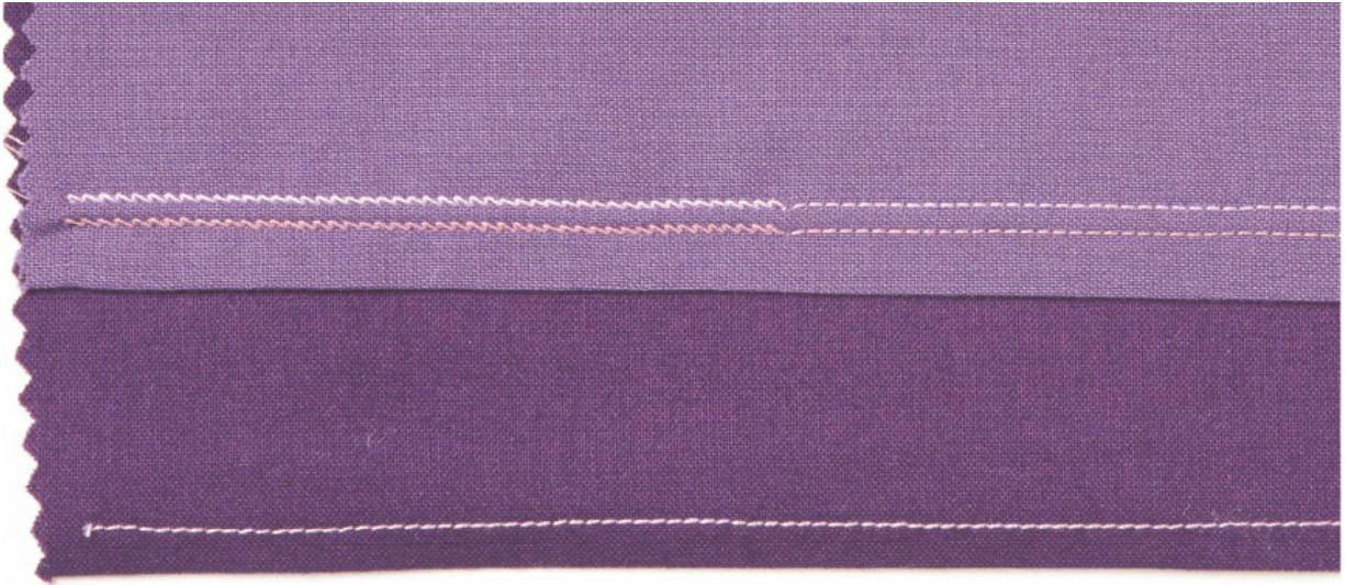
Topstitched hems – twin and narrow stitching
