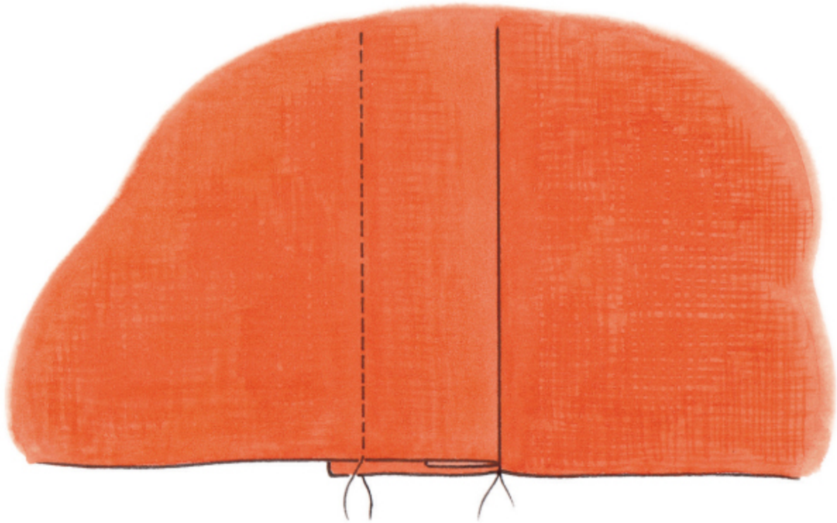
Diagram 4: Encase the trimmed seam allowance
