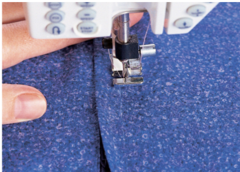
Stitching a lapped zipper from the right side of the garment
